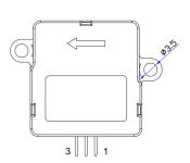
Note: The positioning hole on the manifold that receives the post shall have a diameter between 3.2 and 3.3mm, and a depth greater than 3.3mm. Contact Posifa for sensor CAD model.
