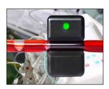
Introtek's AD8/AD9 non-invasive air bubble & air-in-line sensors incorporate the latest ultrasonic technology. Introtek AD8 (for rigid tubing) and AD9 (for soft tubing) sensors incorporate the latest generation of pulse-type ultrasonic circuitry. Integral to the sensor's assembly, the Micro-Electronic Controller (MEC) features programmable algorithms for functionality control. Response times, time delays and other functions are programmable to specific requirements.
